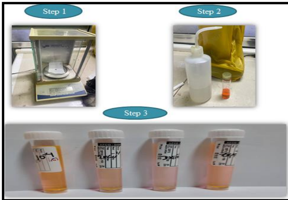
Fig.2. Main steps of R6G dye preparation in the laboratory, including weighing, dilution, and transferring the prepared solutions into labeled tubes.
