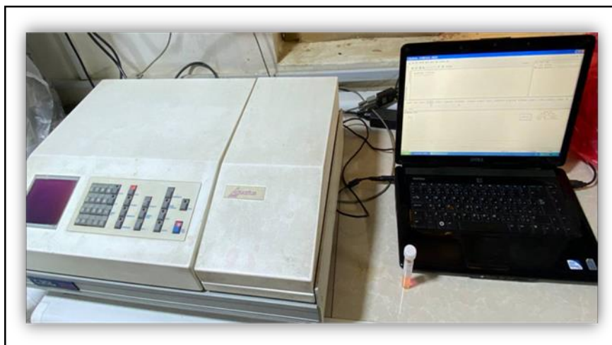
Fig. 4. UV–Vis spectrophotometer used for recording the absorption spectra of \text{TiO}_2 , R6G, and \text{TiO}_2 –R6G hybrid samples.
